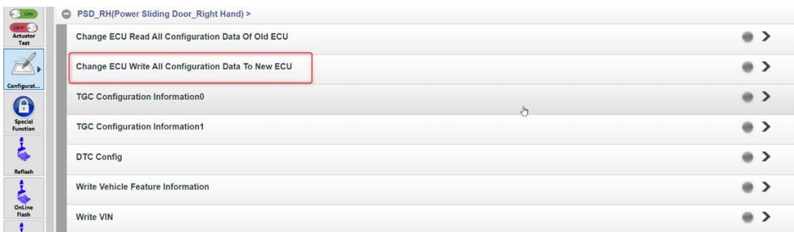
6) After entering the "Change ECU Write All Configuration Data To New ECU" menu, if the ECU operation is only for one vehicle model, please select "Write configuration for this vehicle", as shown in the following figure:
