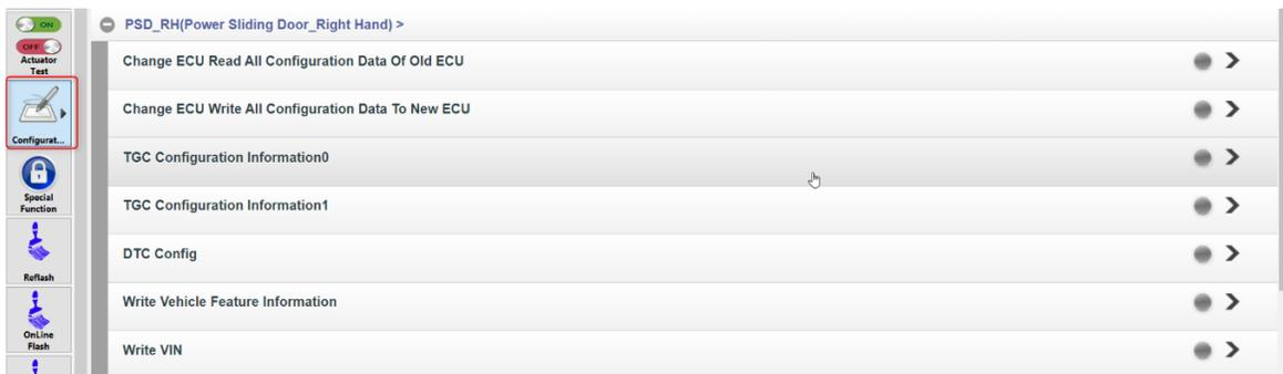
2) 例: For example: select and click on PSD RH (right electric sliding door module) to first read the data of the old ECU. Please click on the **"Change ECU Read All Configuration Data Of Old ECU"** menu, as shown in the following figure:
